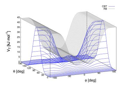
Fig. 5.28: Blue: surface plot of the combined bending-torsion potential ((5.183) with  $k = 10 \text{ kJ mol}^{-1}$ ,  $a_0 = 2.41$ ,  $a_1 = -2.95$ ,  $a_2 = 0.36$ ,  $a_3 = 1.33$ ) when, for simplicity, the bending angles behave the same ( $\theta_1 = \theta_2 = \theta$ ). Gray: the same torsion potential without the sin<sup>3</sup>  $\theta$  terms (Ryckaert-Bellemans type).  $\phi$  is the dihedral angle.
