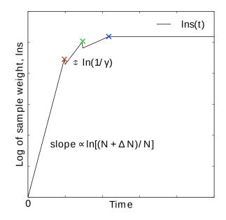
Fig. 5.43: In the final stage, N grows at the sampling rate and thus  $1/N \sim 1/t$ . The exit from the final stage is determined on the fly by ensuring that the effective sample weight s of data collected in the final stage exceeds that of initial stage data (note that  $\ln s(t)$  is plotted).
