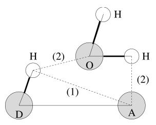
Fig. 5.59: Insertion of water into an H-bond. (1) Normal H-bond between two residues. (2) H-bonding bridge via a water molecule.
