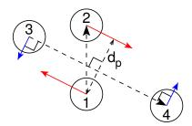
Fig. 5.40: The pull setup for geometry direction-relative. The "normal" pull groups are 1 and 2. Groups 3 and 4 define the pull direction and thus the direction of the normal pull forces (red). This leads to reaction forces (blue) on groups 3 and 4, which are perpendicular to the pull direction. Their magnitude is given by the "normal" pull force times the ratio of  $d_p$  and the distance between groups 3 and 4.
