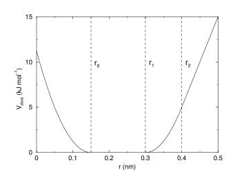
Fig. 5.31: Distance Restraint potential.
