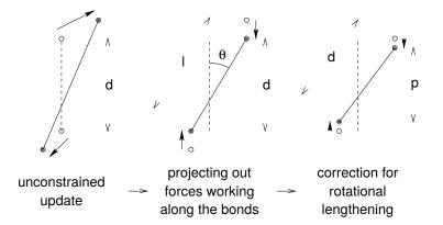
Fig. 5.8: The three position updates needed for one time step. The dashed line is the old bond of length d, the solid lines are the new bonds.  $l = d \cos \theta$  and  $p = (2d^2 - l^2)^{\frac{1}{2}}$ .
