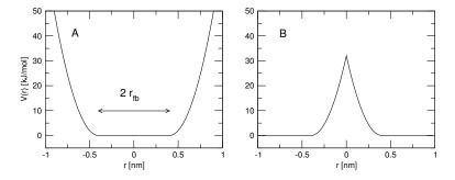
Fig. 5.30: Flat-bottomed position restraint potential. (A) Not inverted, (B) inverted.
