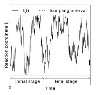
Fig. 5.41: AWH evolution in time for a Brownian particle in a double-well potential. The reaction coordinate  $\xi(t)$  traverses the sampling interval multiple times in the initial stage before exiting and entering the final stage. In the final stage, the dynamics of  $\xi$  becomes increasingly diffusive.
