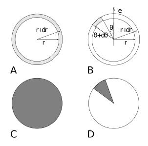
Fig. 5.52: Definition of slices in *gmx rdf* (page 238): A.  $g_{AB}(r)$ . B.  $g_{AB}(r, \theta)$ . The slices are colored gray. C. Normalization  $\langle \rho_B \rangle_{local}$ . D. Normalization  $\langle \rho_B \rangle_{local, \theta}$ . Normalization volumes are colored gray.
