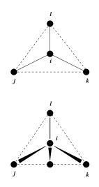
Fig. 5.24: Principle of improper dihedral angles. Out of tetrahedral angle. The improper dihedral angle  $\xi$  is defined as the angle between planes (i,j,k) and (j,k,l).
