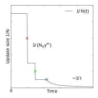
Fig. 5.42: In the final stage, the dynamics of  $\xi$  becomes increasingly diffusive. The times of covering are shown as  $\times$ -markers of different colors. At these times the free energy update size  $\sim 1/N$ , where N is the size of the weight histogram, is decreased by scaling N by a factor of  $\gamma = 3$  (note that the default value of  $\gamma$  is 2 since GROMACS 2024).
