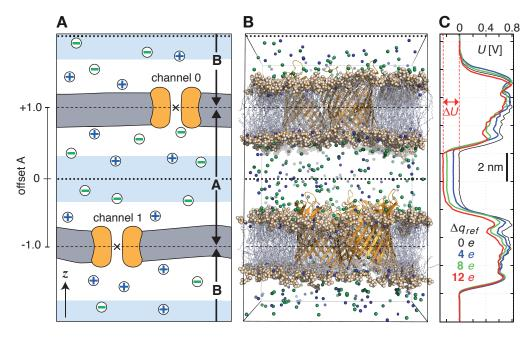
Fig. 5.49: Typical double-membrane setup for CompEL simulations (A, B). Ion/water molecule exchanges will be performed as needed between the two light blue volumes around the dotted black lines (A). Plot (C) shows the potential difference  $\Delta U$  resulting from the selected charge imbalance  $\Delta q_{ref}$  between the compartments.
